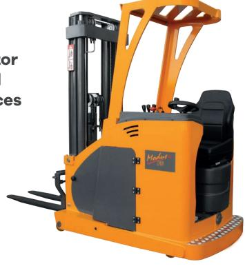
The Modus FS ac forklift trucks with counterweight, operator seat and tilting forks are ideal for special load handling over long distances. Lateral steering wheel for optimal visibility on aisles, in both directions. Rugged structure for maximum reliability in extreme conditions. Characterised by compact size and high manoeuvrability, suitable for applications in all sectors. For lifting between 1,610 mm and 4,610 mm.
