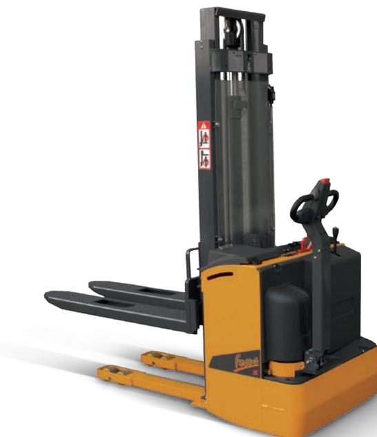
The battery compartment can be easily opened by lifting the hinged cover, simplifying the daily and periodical battery recharge and check operations. The Focus ac is available with batteries of up to 375 Ah. With the wo-wa battery charger installed on-board (optional) you can recharge your truck from any socket.
