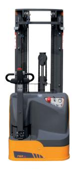
Facilitated maintenance operations thanks to wide chassis opening that allows replacing the drive wheel without lifting the entire truck. New polyethylene casings with innovative opening system for easy access to all main components during routine and extraordinary maintenance operations.
