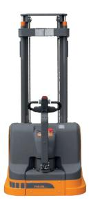
The mini joystick (finger touch) allows the operator to control the truck by simply moving his finger along the tiller, ensuring precise and smooth load lifting and lowering, without taking his hands off the tiller. The electronic control comes with IP 65 protection rating and is waterproof and dustproof. The tiller head can also be manufactured with IP55 protection rating for protection against dust and water (standard feature for cold store versions).
