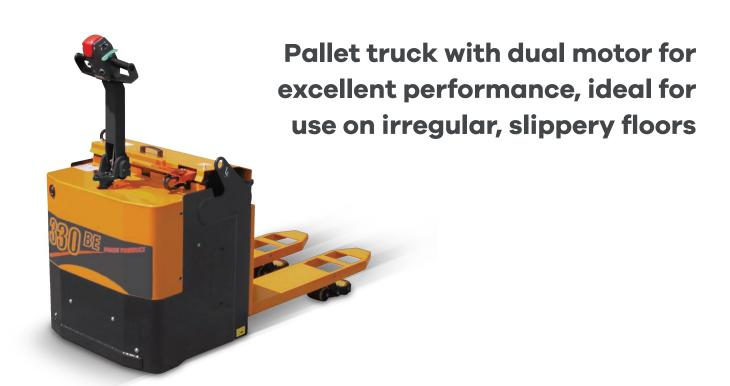
The 330 BE dual motor electric pallet trucks are ideal for use on irregular and slippery floors. Equipped with a dual wheel drive system connected to a servo-assisted tiller that ensures the power necessary for the truck to overcome any bumps, ensuring optimal driving comfort.
