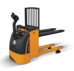
The 316 KN-C and 316 KN-M pallet trucks with mast combine the traditional pallet truck function with the ability to store the load at various height levels. Ideal for safe and comfortable manual load picking and storage in small spaces and on narrow paths, also suitable for overlapped loads.
